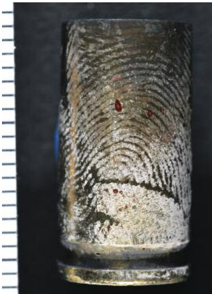
Friction ridge impression developed on a 9 mm bullet casing from an attempted murder using cyanoacrylate fuming.
